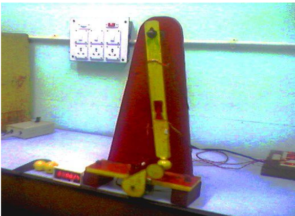
Fig 5 Experimental setup for impact fatigue testing
